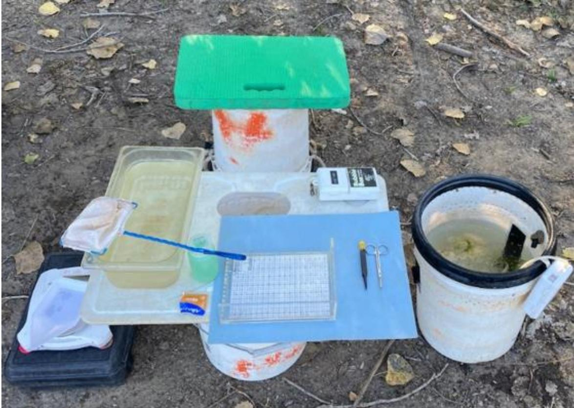
**Figure 5: Fish processing station consisting of an anesthetic tank, 5-gallon recovery bucket, digital scale, measuring board, and genetic sampling equipment.**
